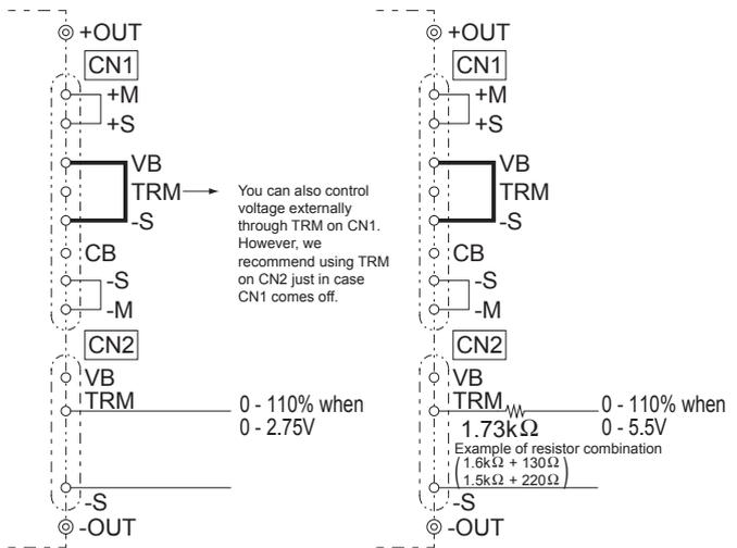
Fig.2.1 Wiring 1
