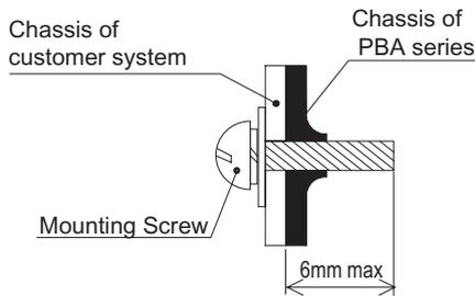
Fig.5.1 Mounting screw
