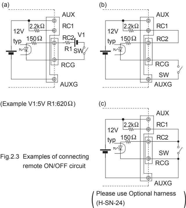
Fig.2.3 Examples of connecting remote ON/OFF circuit
