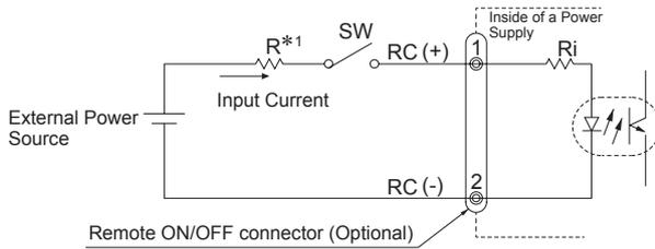
Fig.7.7 Example of using a remote ON/OFF circuit
